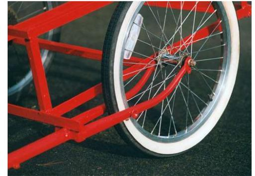
The next part is the towing bar. It needs to line up exactly with the left hand rear wheel mount.
