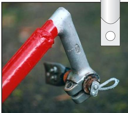
To strengthen the joint, weld or bolt the stem in place. Two bolts will be needed to prevent the towing arm from twisting.
